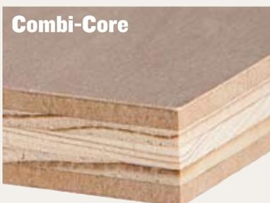
**Combi-Core Panels** Constructed of veneer core inner plies with particleboard or MDF crossbands. Offers similar strength and stability to veneer core but has the void-free surface quality of PBC or MDF. Excellent substrate for thin sliced woods and rotary woods, reducing the potential for core transfer. Combi-core panels, like ClassicCore™, tend to offer more consistent tolerances than standard veneer cores.
