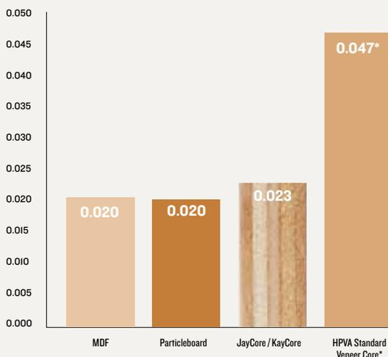
\*The above ranges refer to the data collected in the plywood comparison test. Compare this to the ANSI/HPVA-HP-1-2004 standard which permits a tolerance of +0-0.047” for panels 1/4” and thicker.
